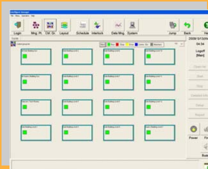
The Control Group list further categorizes equipment into partitions including individual buildings, entire floors or specific areas. Operational status can be determined at a glance.
