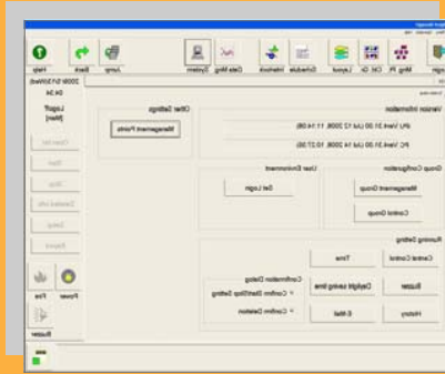
The Control Group further categorizes equipment into partitions like individual buildings, floors or specific areas. Operational status can be determined at a glance.
